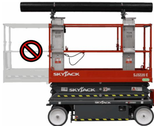
*The holder is divided into two - an upper and a lower part. Mount the lifting column in the upper part.*
