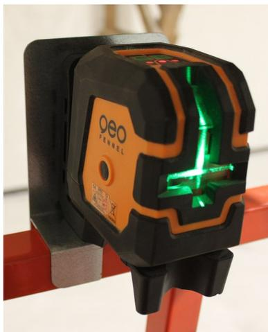
If you are using a (magnetic) line laser, place the supplied holder on the railing of the lift. So far, the holder only fits railings on Skyjack lifts.
